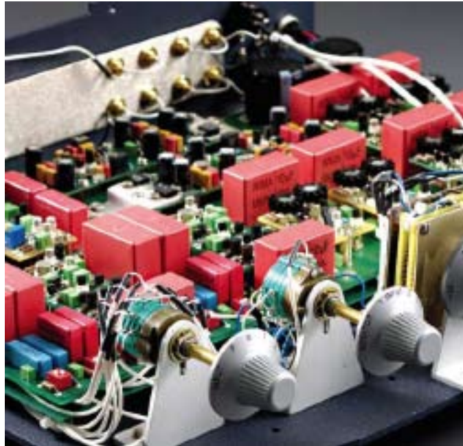
Internal view of Cello Preamp. It's easy to notice the components quality: capacitors of signal coupling and power supply decoupling are made by WIMA and they belong to the polypropylene series (MKP) much better than the MKT series in polystyrene.
