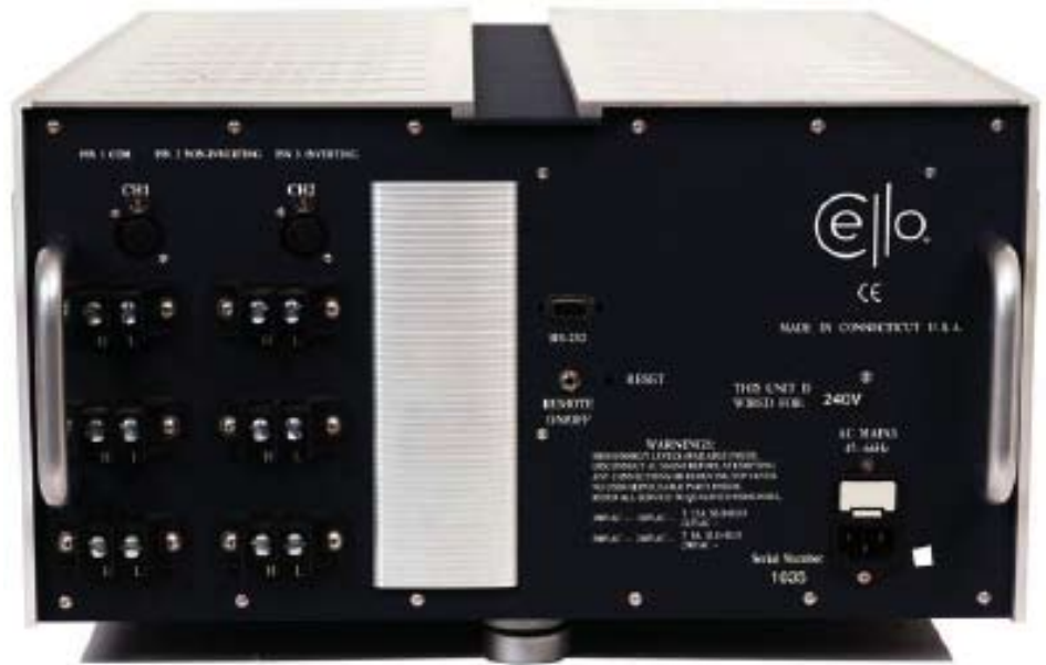
On the Rhapsody back at the left the 3 channel outputs are realized to accept only bare cable blocked with it's screw.. At the centre the RS 232 link.
