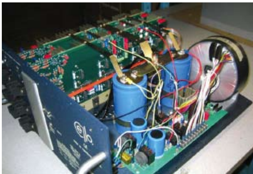
Internal view of the Cello Power Amp. You can see the toroidal transformer, the filtering electrolytics, remarkable the great bars to deliver the high alimention currents into the amplification SHEDE. A remark also for the cooling section hosting the power transistors: Cello deliberately choose a complex mounting technique, consequently a costly one, which delivers many sonic advantages.
