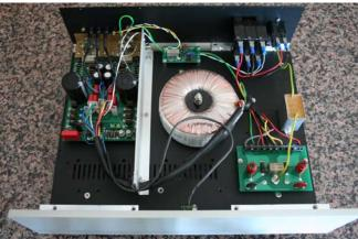
As is our standard practice, we've taken the covers of the Encore amplifier and Master power supply to have a look. You will immediately notice that these are not individual mono units, but rather a separation of amplifier channels and regulated power supply.
