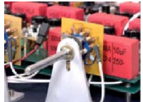
Switches with fixed resistors serve as gain controls for balance.
