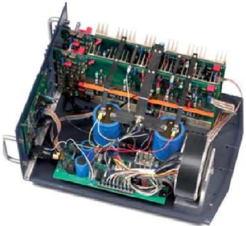
One power supply feeds both channels in the Rhapsody.
